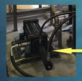
Model VRH400/10/1250 with 45kW hydraulic pack, work simultaneously with Polymer dosing, a hydraulically driven slave polymer dosing system
