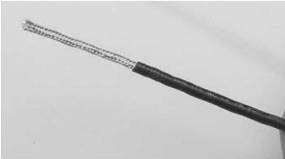
Figure 3.2 – Removing outer plastic jacket
