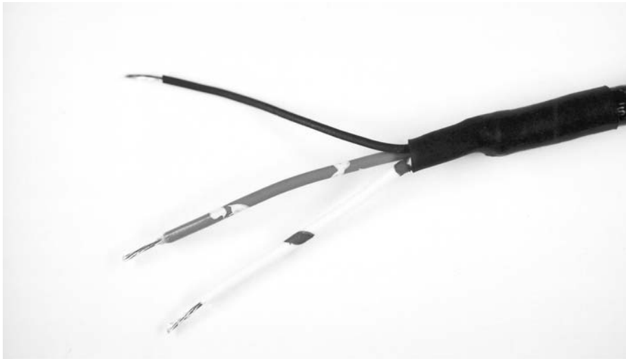
Figure 3.5 – Applying heat shrink tubing
